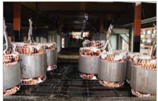
Automatic Impregnation Plant
